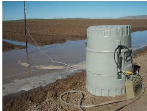
*Plate 1: ISCO water sampler.*
