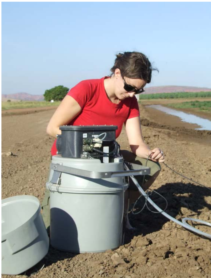
Fiona Tingle setting up the automated water sampler on farm in 2008
