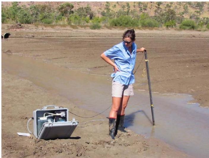
New Environmental Officer for the Ord Irrigation Cooperative Anna Price installing an automatic sampler in a farm tail drain.
